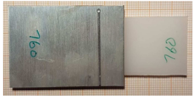
Figure 5. Plan view of the laser beam joint between aluminum and polyamide 6.6.
